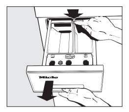
■ Pull out the detergent dispenser drawer until a resistance is felt. Press down the red release catch and at the same time pull the drawer right out of the machine.
